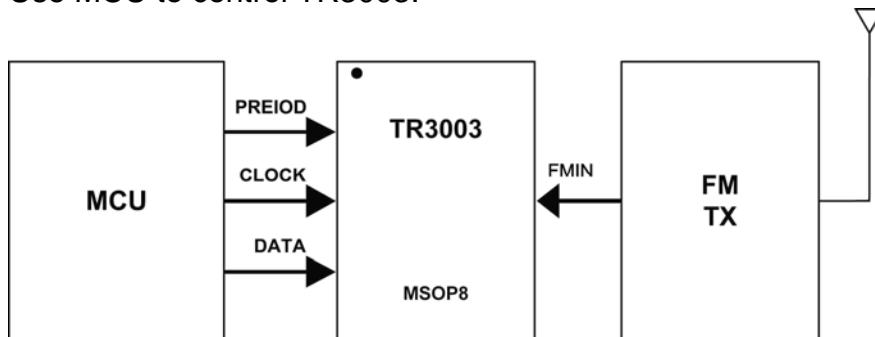
(9). The following program example uses the 4 bit MCU of tenx technology inc. to control TR3003 and transmit 87.0MHz [1AD4(hex)] FM frequency signal. (Use IOA port to transmit PERIOD & CLOCK & DATA signals. And define IOA3=PERIOD & IOA2=CLOCK & IOA1=DATA)
