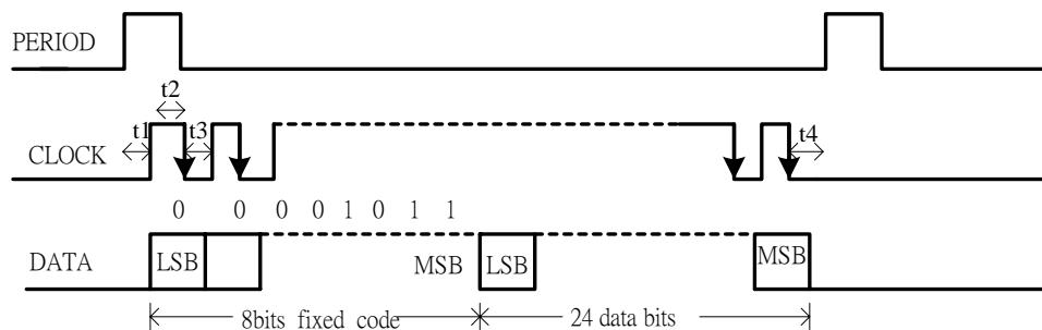
**(A). PERIOD signal:** Between the two PERIOD signals (upward edge to upward edge), there shall be 32 CK clocks included.
