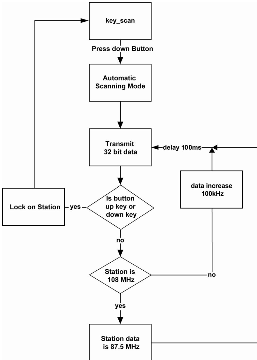
(2). Flow diagram mode to replace 0.1MHz transmission frequency each time:
