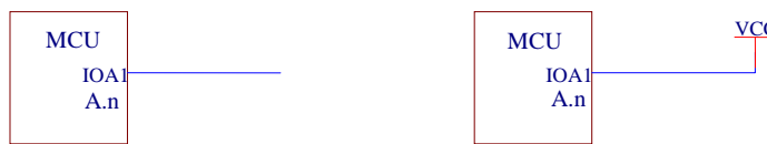
Fig. 2 Use the input pins with the pull down resistor for bonding option
