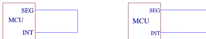
Fig. 3 Use external pin INT and output pin with SEG wire for bonding option
