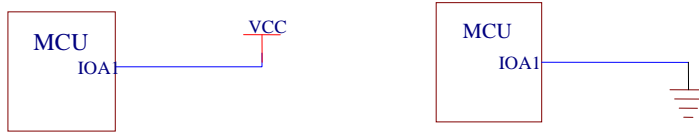
Fig.1 Use the input pins without the pull down resistor for bonding option
